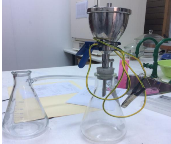
14(A) – Total Contamination Set-up
