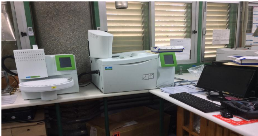
3(A) – Free& Total Glycerin Test Set-Up
