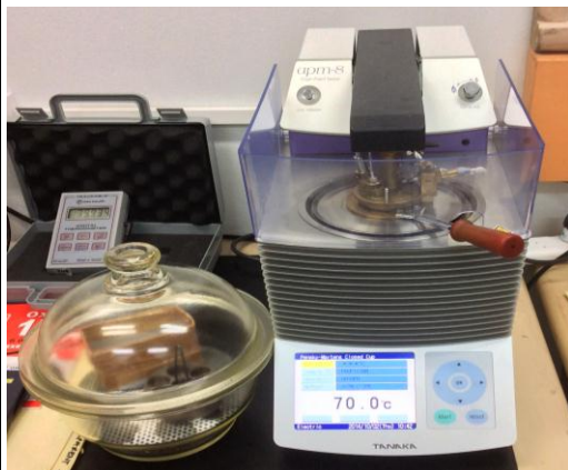
7(A) – Automated Canon Pensky-Martens Closed Cup Tester
