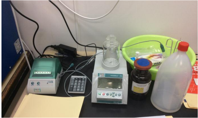
13(A) - Automatic Coulometric Karl Fisher Titrator.
