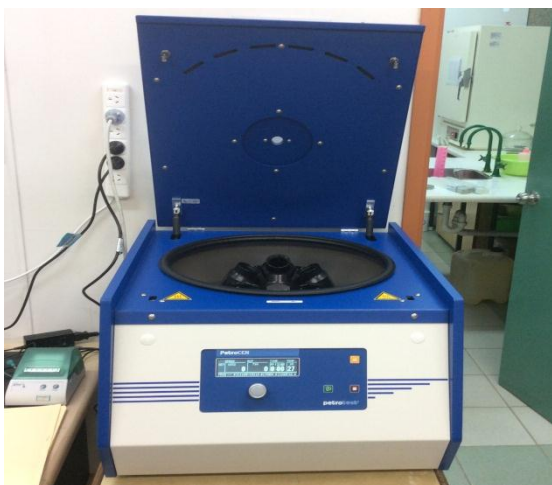
9(A) – Centrifuge Used in Water & Sediments Test Method
